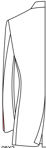
C-05X2 sleeve slit big middle stitch sleeve slit 0.6cm 0.15 narrow external pick stitch
