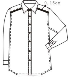
S-531S S-532B front style:0.3cm contrast in shoulder
