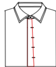
520C outer folded placket with knots of 3cm top & 3.7cm bottom with appointed fabric-
