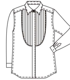
5039-Front style:Front U shap, 6 pleat of 1.3cm for each side
