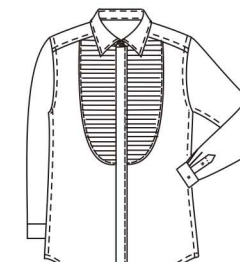
5B26-front piece tuxedo patch with horizontal pleats, to front fly's fourth button(not counting the collar button), 1cm width pleats, 0.4cm pleat distance,with piping
