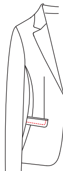
15D6 Lower pocket with 0.8 top stitching
