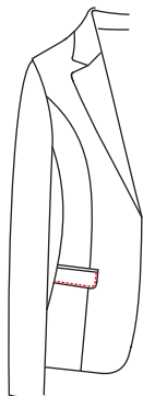
15D4 Lower pocket with 0.15 top stitching
