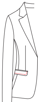
15D5 ↩ Lower pocket with 0.6 top stitching
